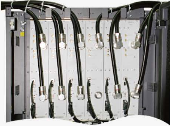
Connections of RF jumpers for a single cabinet
